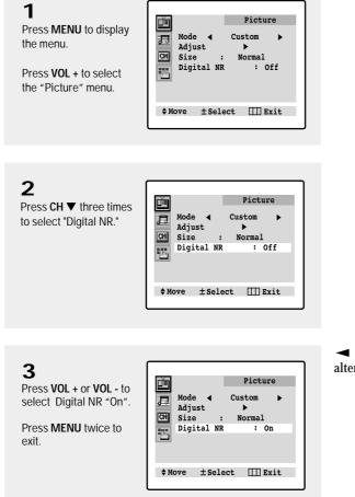
◄ Pressing VOL- or VOL+ will alternate between "On" and "Off".
